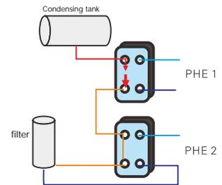
PHE application in condensing liquid purifying
