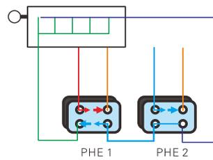
PHE application in diesel oil cooling
